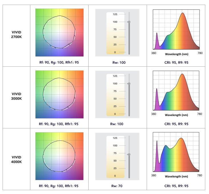
Rf: TM-30 metric measuring color fidelity (whether colors are similar to those under natural light). Rf is a more accurate version of the CRI Ra. Rf is 100 for natural light. Rg: TM-30 metric measuring color gamut (whether colors are more saturated than under natural light). Rg is 100 for natural light.
