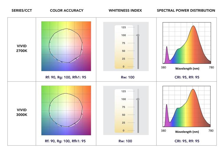
Rf: TM-30 metric measuring color fidelity (whether colors are similar to those under natural light). Rf is a more accurate version of the CRI Ra. Rf is 100 for natural light. Rg: TM-30 metric measuring color gamut (whether colors are more saturated than under natural light). Rg is 100 for natural light. Rfh1: TM-30 metric measuring color fidelity for red tones. Rfh1 is a more accurate version of the CRI R9. Rfh1 is 100 for natural light.
